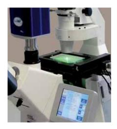
Multi color imaging with automatic color detection and overlay up to seven fluorescence channels per well gives the user a high flexibility in cellular research. The VisiView® software helps with easy device control and intuitive handling of the software. The macro interpreter language covers all functions for automation for customized automation according to your experimental demands.
